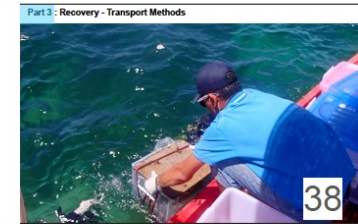
Carefully bring the ARMS onto the boat and to the holding buckets, flip the ARMS so it is upright in the holding buckets and transfer all water and sediment from the transfer buckets into the holding buckets
